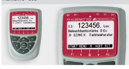
ALMEMO® professional measuring instrument, latest V7 generation with data logger function Two measuring inputs for all digital ALMEMO® D6 and D7 sensors, for ALMEMO® standard sensors with the DIGI measuring range. Special functions for applications using ALMEMO® D7 sensors
